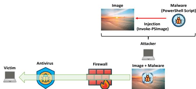
**Figure 1:** Reference attack model: an attacker embeds a malicious script into an innocent-looking image to evade detection and security tools.
